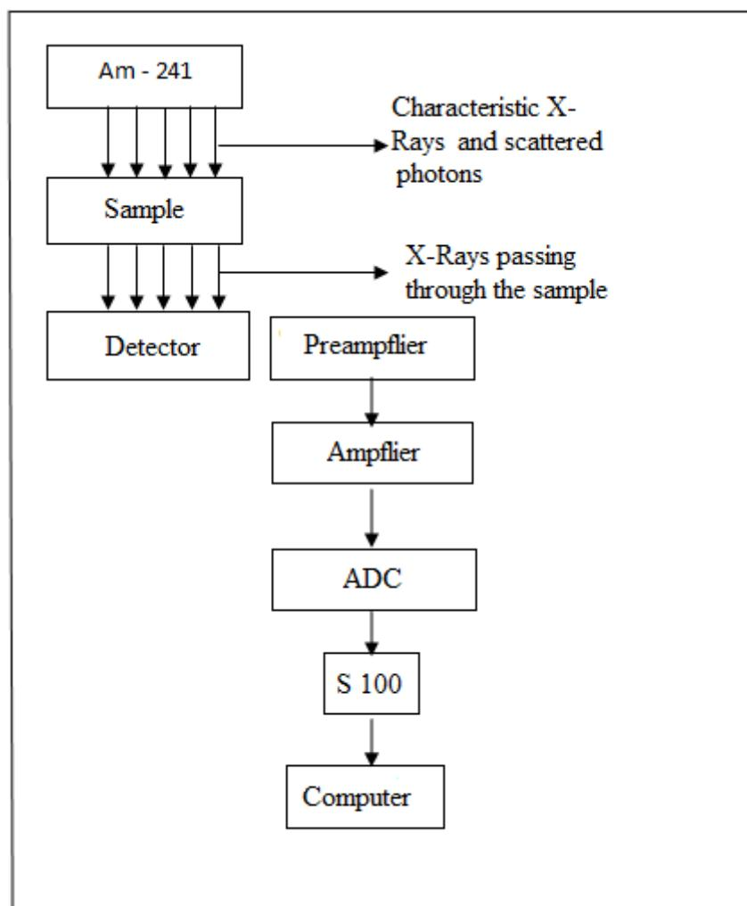
**Figure 1.** Radiation Absorption Scheme
