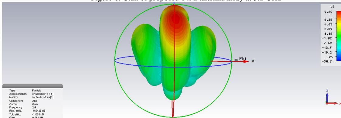
Figure 7. Gain of proposed 2 x 2 array antenna at 2.4 GHz
