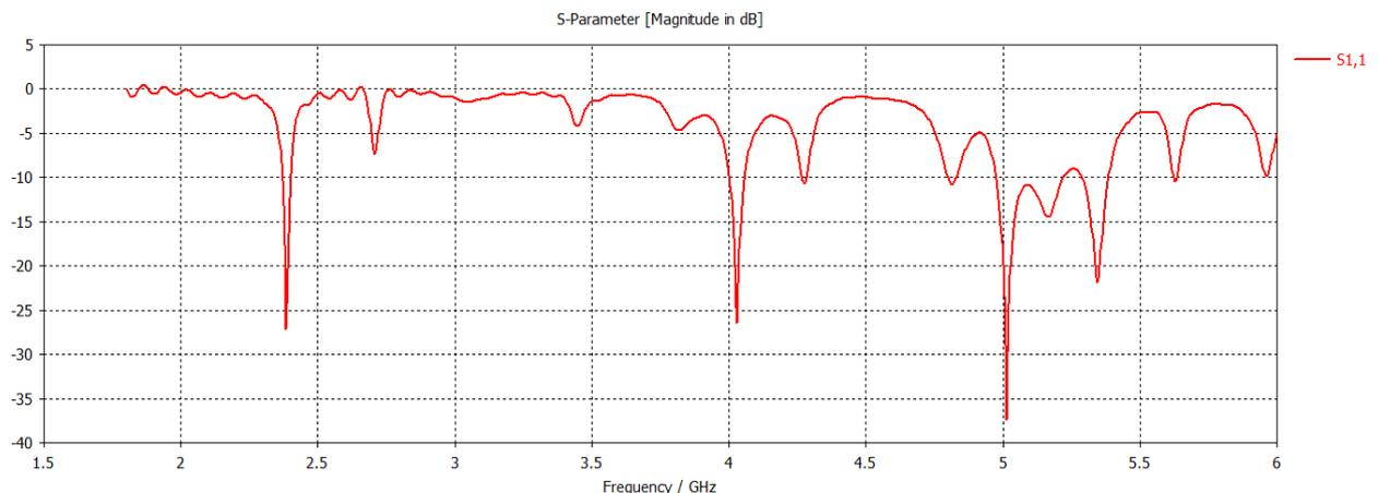
Figure 4. Return loss of 2 x 2 array antenna
