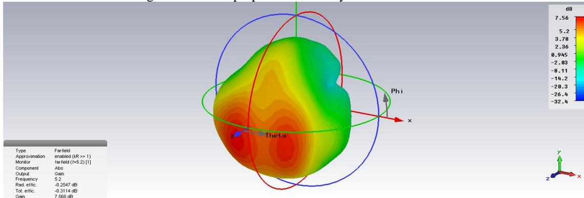
Figure 6. Gain of proposed 1 x 2 antenna array at 5.2 GHz
