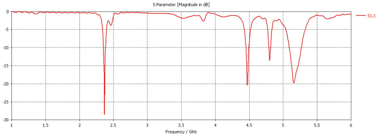
Fig 3: Return loss of 1 x 2 array antenna
