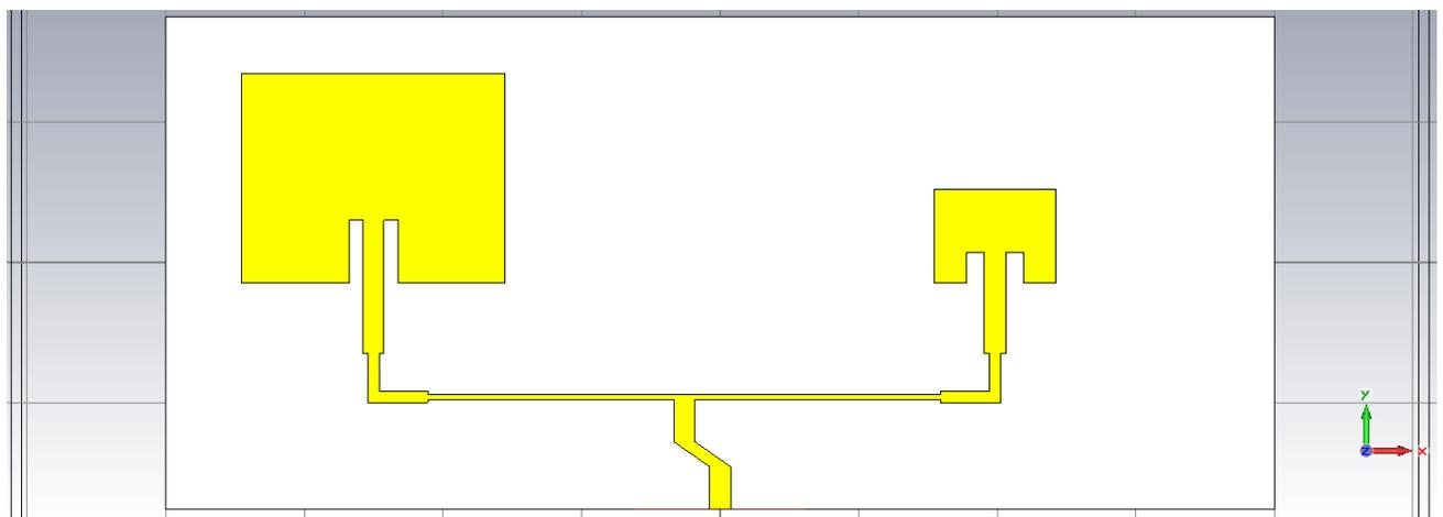
Figure 1. 1 x 2 array antenna
