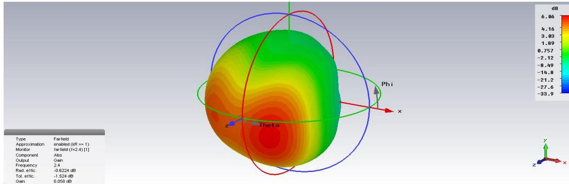
Figure 5. Gain of proposed 1 x 2 array antenna at 2.4 GHz
