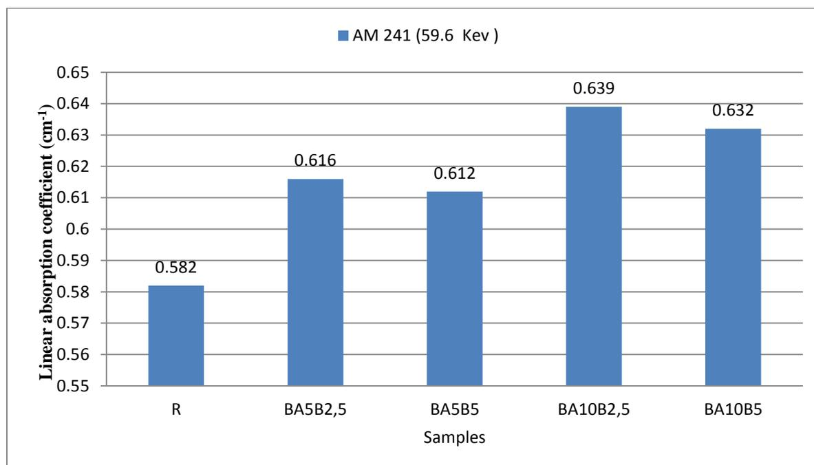
**Figure 6.** Linear absorption coefficient of barite, cholemanite and wheat stalk doped specimens
