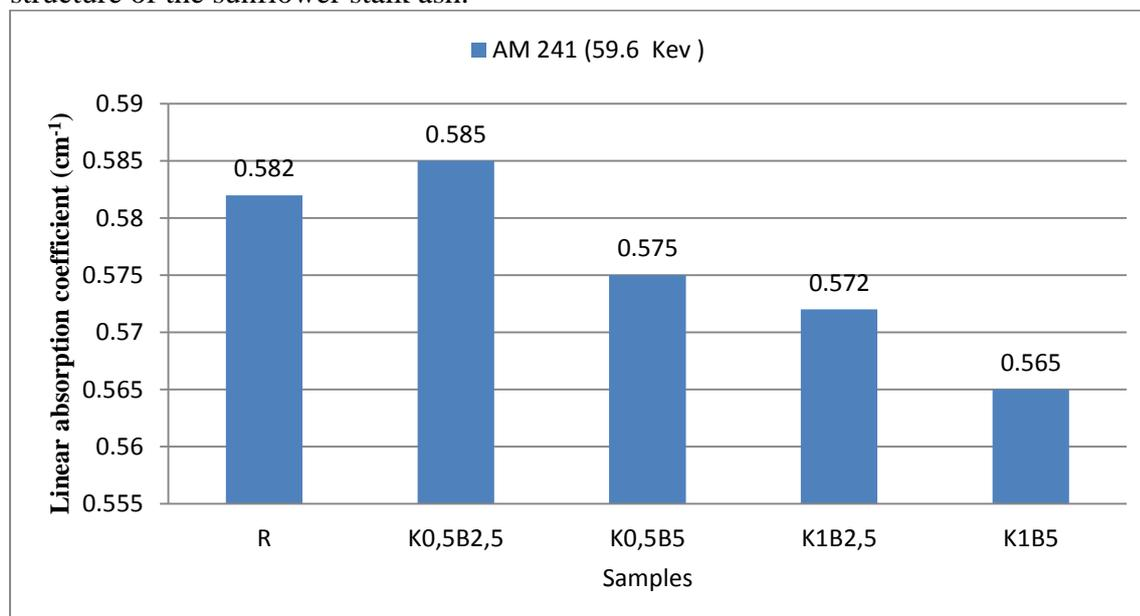
**Figure 5.** Linear absorption coefficient of barite, cholemanite and wheat stalk ash doped specimens
