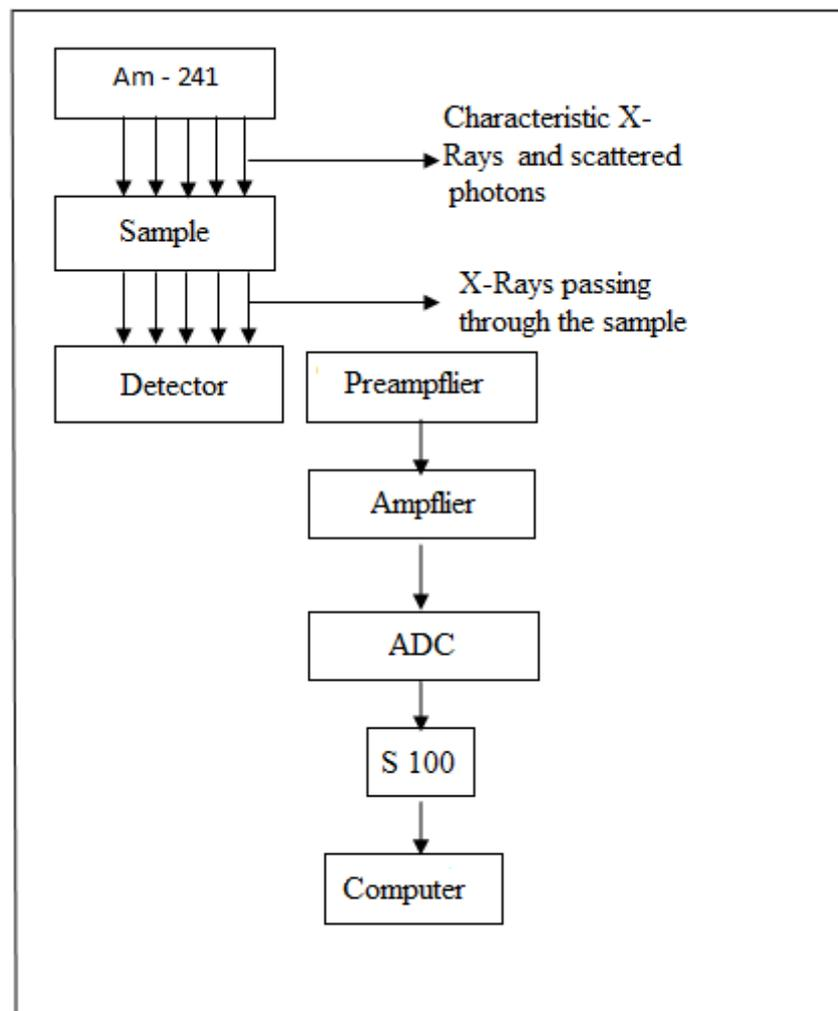
**Figure 1.** Radiation Absorption Scheme
