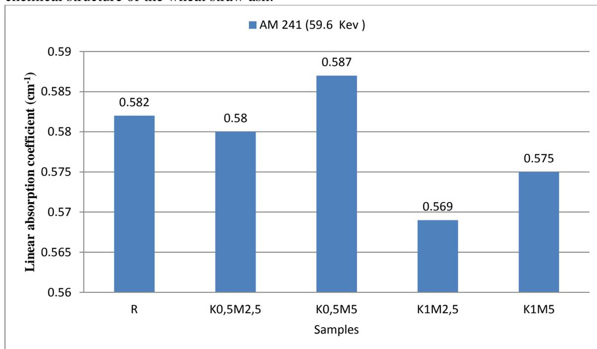
**Figure 7.** Linear absorption coefficient of barite, cholemanite and corn stalk doped specimens
