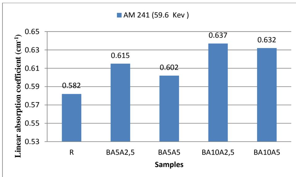
**Figure 3.** Linear absorption coefficient of barite, cholemanite and sunflower stalk ash doped specimens
