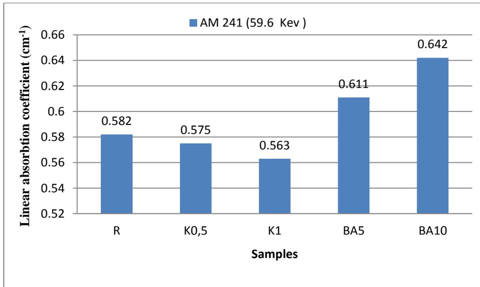
**Figure 2.** Linear absorption coefficient values of barite and cholemanite doped samples
