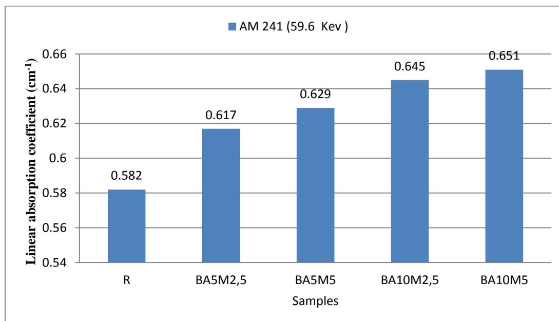
**Figure 8.** Linear absorption coefficient of barite, cholemanite and corn stalk doped specimens
