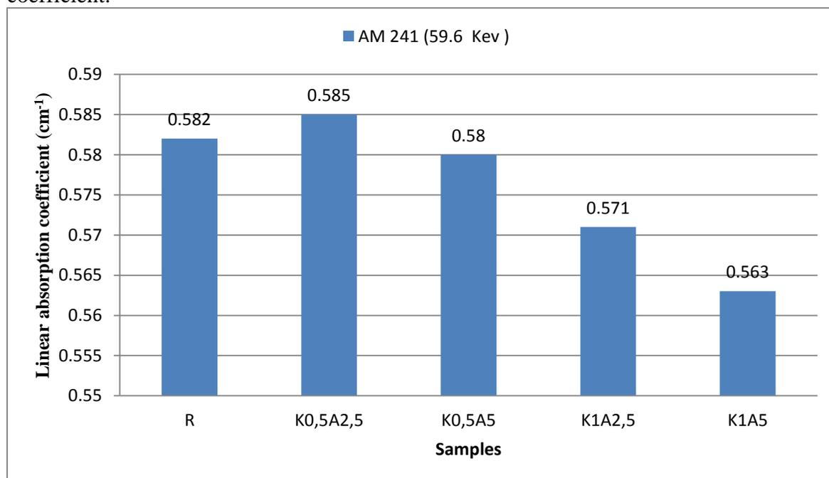
**Figure 4.** Linear absorption coefficient of barite, cholemanite and sunflower stalk ash doped specimens
