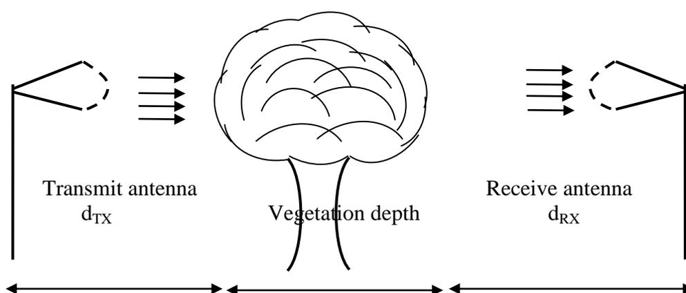
**Figure 1.0 Link configuration for isolated tree measurement**
