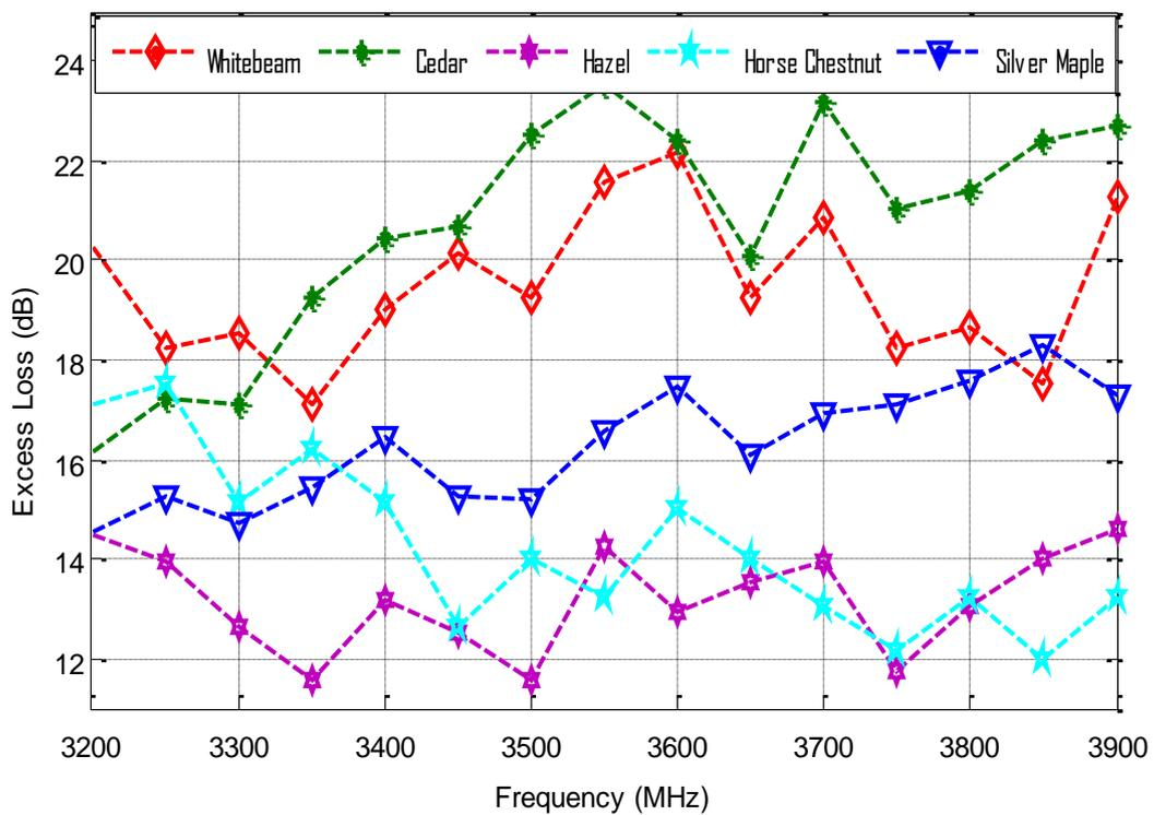
Figure 3a. Excess Loss across different trees at 3.2 – 3.9 GHz
