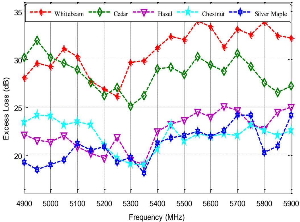
Figure 3b. Excess Loss across different trees at 4.9 – 5.9 GHz
