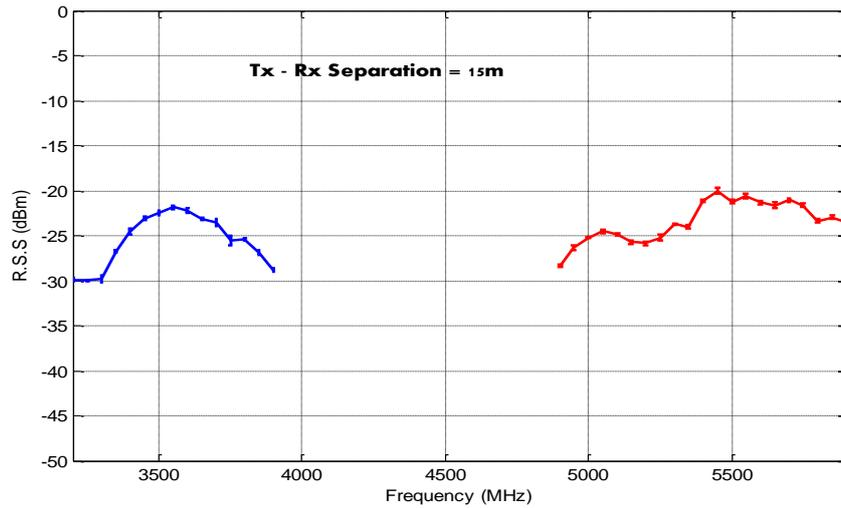
Figure 2.0 Free space R.S.S versus frequency for a fixed distance at 3.5 and 5.4 GHz bands.
