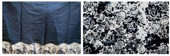
Fig., 13: Discharge effect produced only at the edge of the fabric with lace material
