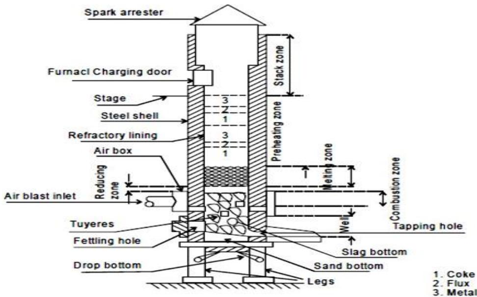
Figure 2: Sectional view of the cupola furnace
