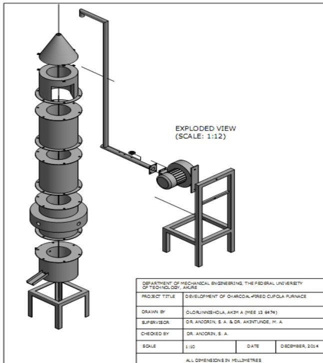
Figure 1: An exploded view of the fabricated erythrophleum suaveolens charcoal-fired cupola furnace.
