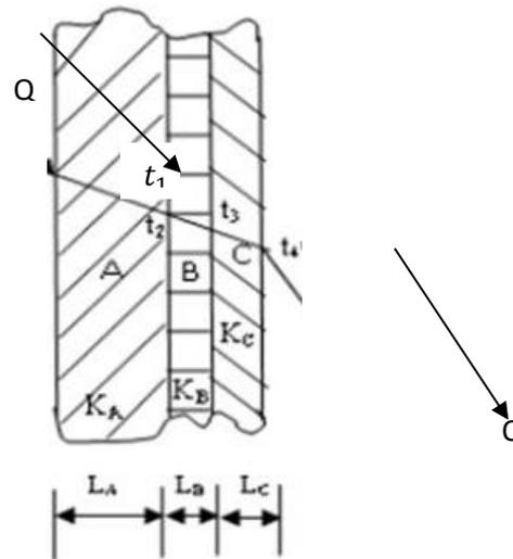
Figure 4: Heat conduction through the furnace.
