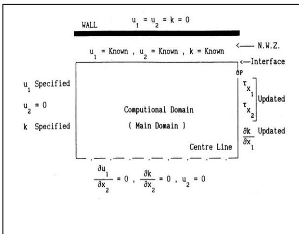
Fig.1 Boundary conditions when the mesh is terminated at small distance away from the wall N.W.Z.
