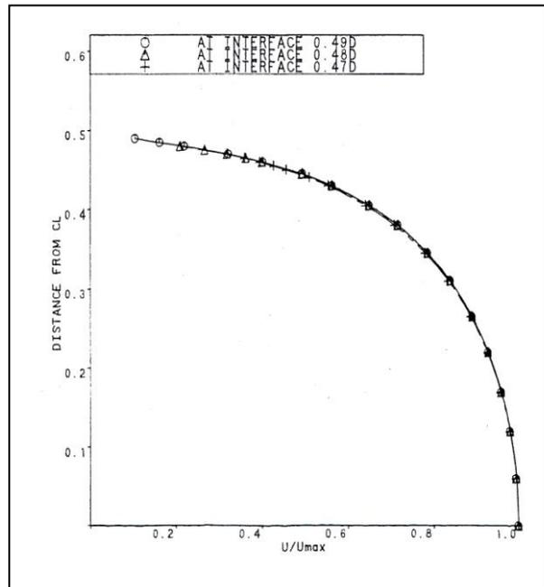
Fig. 4 Developing velocity profiles, solved in one matrix
