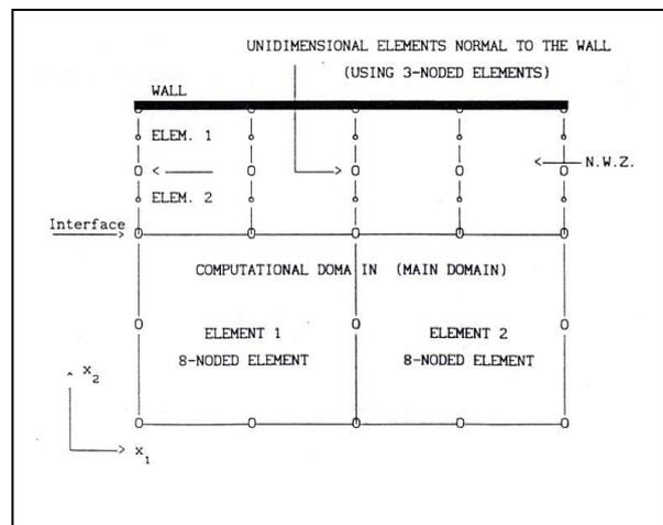
Fig. 2 One-dimensional elements in one-direction normal to the wall used in the
