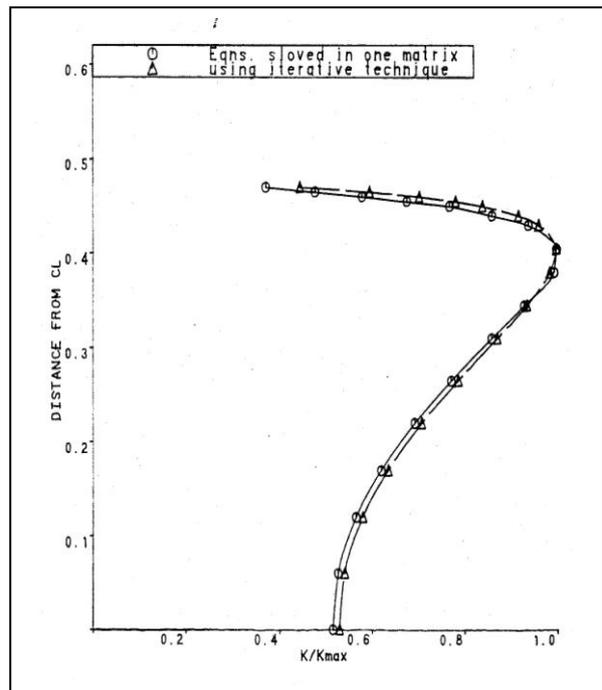
Fig. 6 Downstream kinetic energy profiles for developing turbulent flow when coupled and uncoupled methods used
