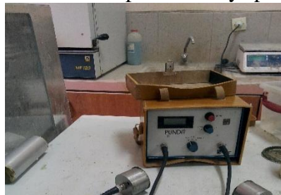
Fig. 8. Ultrasonic pulse velocity measuring device
