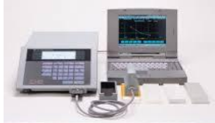
Fig. 7. Thermal conductivity measuring device
