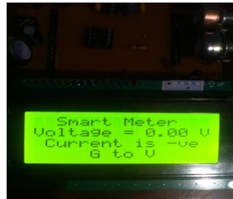
Fig 7. Smart meter shows current direction; G2V
