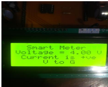
Fig 6. Smart meter measuring voltage and current direction; V2G
