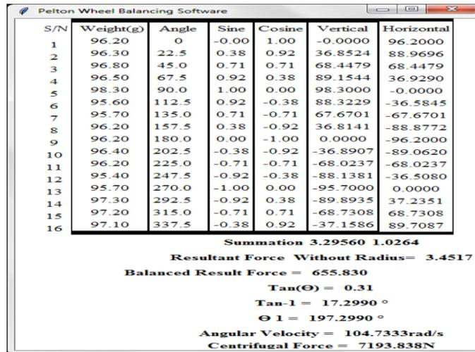
Figure 5: GUI Output display for Sixteen (16) Pelton Cup Selected.
