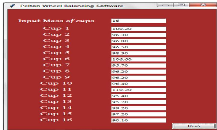
Figure 6: Automatically Generated GUI for Pelton Cups with Out of Control Masses
