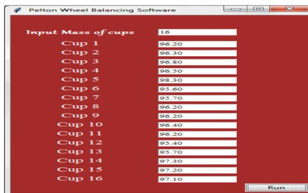
Figure 4: Automatically Generated GUI for Pelton Cups with Statistically Selected Masses.
