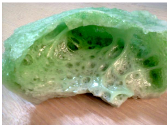
Fig. 4 Internal morphology of the sample directly heated on the microwave reactor
