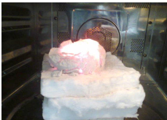
Fig. 3 The direct microwave heating test of the powder mixture based on waste glass on the adapted domestic microwave oven
