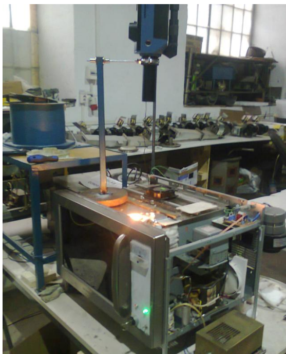
Fig. 1 Adapted 0.8 kW domestic microwave oven
