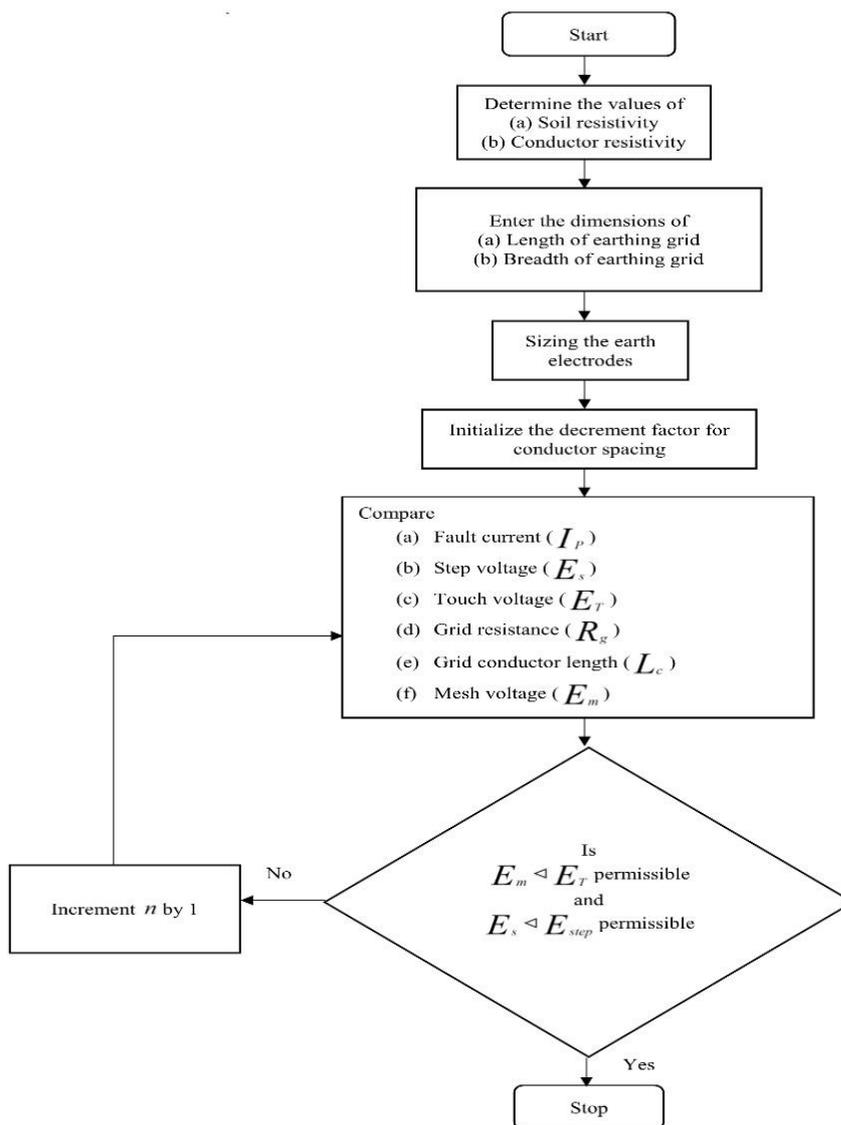
Figure 4. Algorithm for designing a grounding system for a typical A.C. Substation [Arjunsingh et al., 2012; Ubeku and Odiase, 2009]
