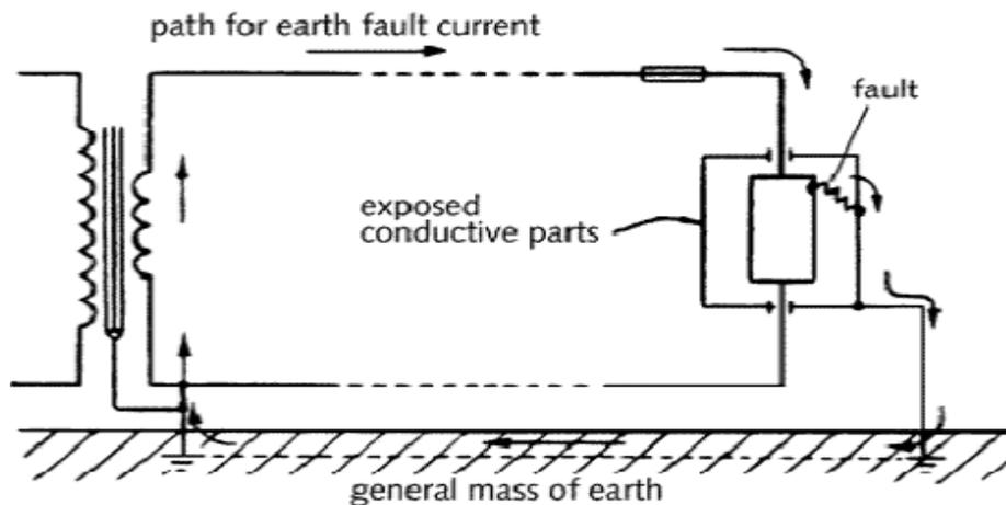
Figure 2. Path for earth fault current (shown by arrows)
