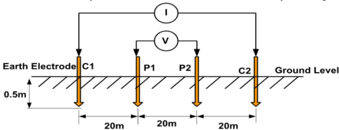
Figure 3. The Wenner Four-Pin Method
