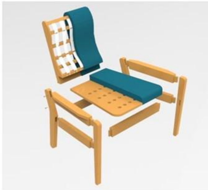
Figure 6: Illustration of the exploded view of the new office chair to be produced for Kumasi Technical University administrative staff
