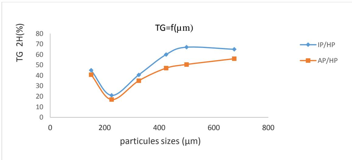
Figure 6: Variation in thickness swelling rates versus particle sizes of cattle horn sheaths during 2H and immersion in water
