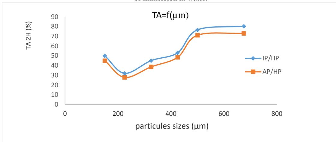
Figure 8: Variation in water absorption rates according to particle sizes of cattle horn sheaths during 2 hours immersion in water.
