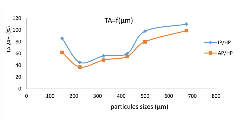
Figure 9: Variation of water absorption rates according to particle sizes of cattle horn sheaths during 24 hours of immersion in water.
