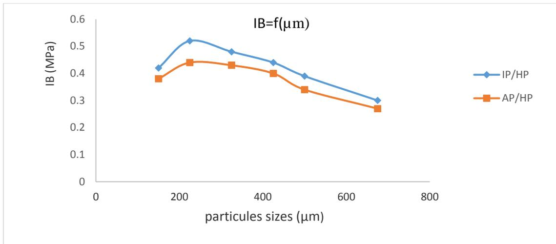
Figure 4: Variation of internal bond according to particle sizes of cattle horn sheaths
