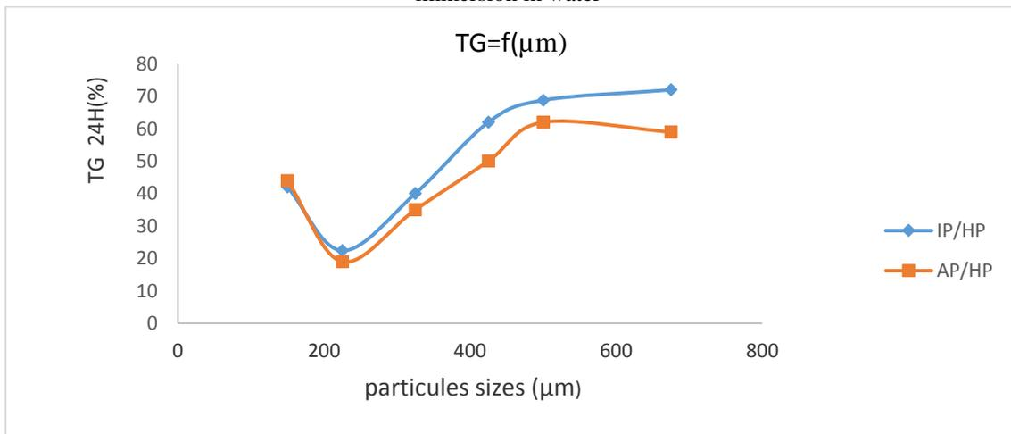
Figure 7: Variation in thickness swelling rates as a function of particle sizes of cowhide sheaths during 24 hours of immersion in water.
