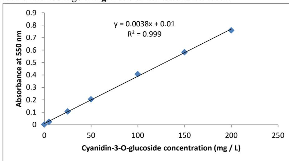
Fig. 2. Calibration curve: Absorbance at 550 nm of different concentrations of cyanidin-3-O-glucoside
