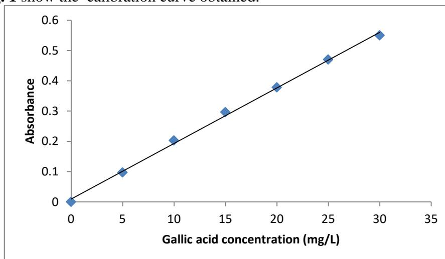
**Fig. 1.** Calibration curve: absorbance at 760 nm of different concentrations of Gallic acid
