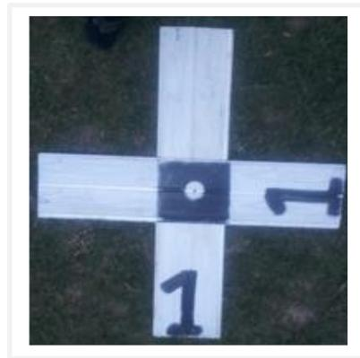
**Figure 2:** Ground Control Point (GCP no.1, 75cm x 75cm)
