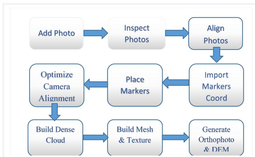
**Figure 5:** Digital Photogrammetric Workflow for Image Processing
