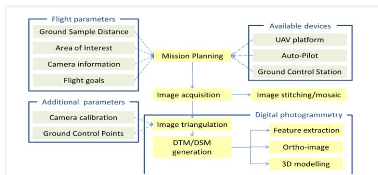
**Figure 3:** Project methodology with UAV photogrammetry
