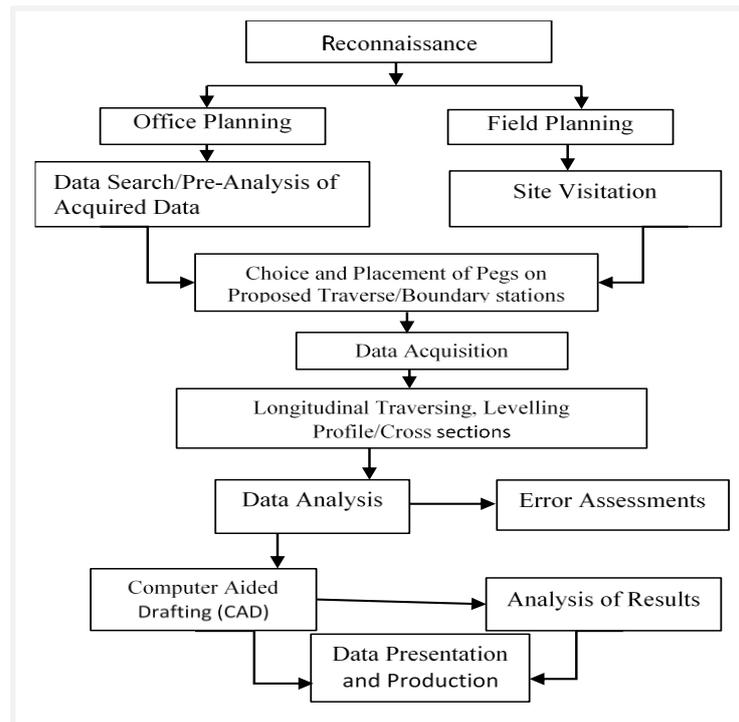
**Figure 4:** Project Methodology with Ground Surveying
