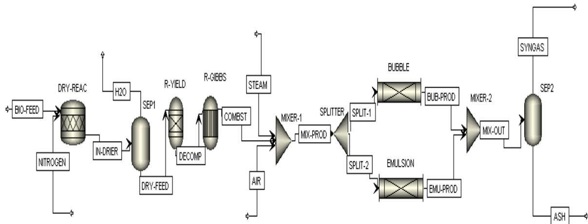
Figure 1: Flow sheet description of the gasification process
