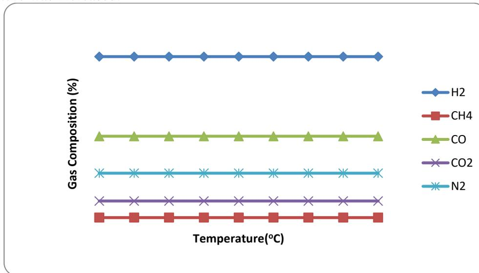
Figure 4: Effect of Gasifier temperature on Syngas composition
