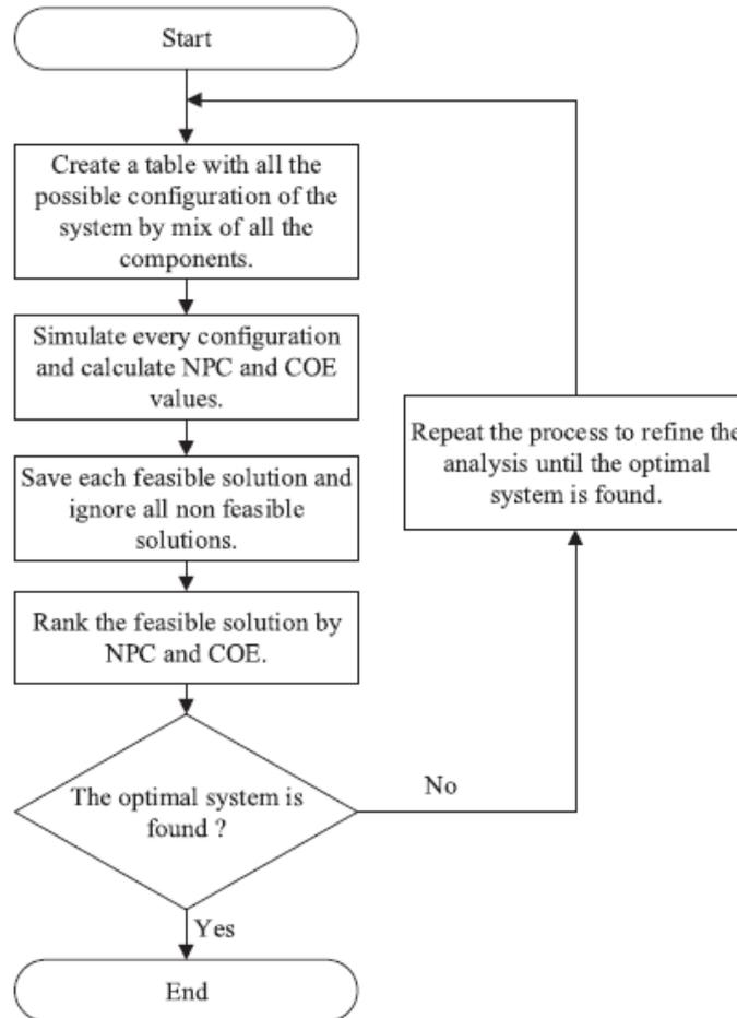
Figure 4: Flowchart of the overall optimisation process (Samir, 2020)
