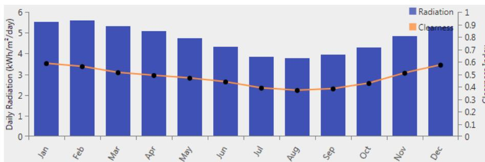
Figure 8: Monthly solar radiation and clearness index (Homer Pro (2017))
