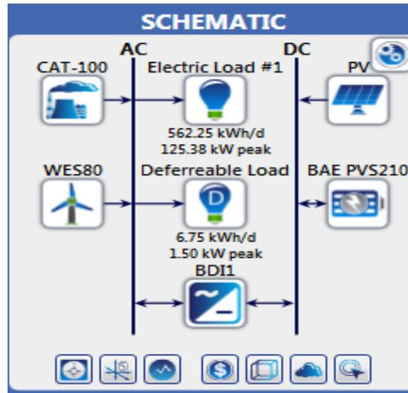
**Figure 9: HRES configuration components (Homer Pro, 2017)**
